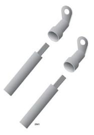
Figure 133. Attaching the Power Wires to the Right Angle Terminals
